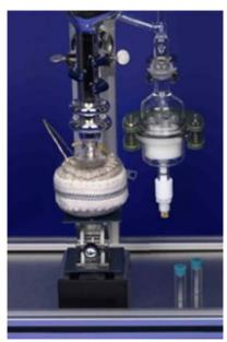
The distillation equipment requires cooling for the column condenser. Cold tap water can be easily attached to the column's condenser. B/R offers heated and refrigerated recirculating baths for more precise control of the condenser temperature.
