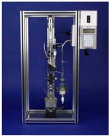
This high efficiency, micro fractional distillation system is an ideal tool for automatically purifying or analyzing a wide range of materials where only very small amounts of sample are available. Common applications include:
