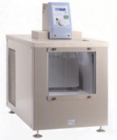
The cover of the bath has four, round, 51 mm holes with lids, for suspending glass capillary viscometers in holders. A permanent light is located in the top plate ensuring optimal visibility. The TV12LT requires only 15 liters of bath medium. A bath overflow outlet protects against expanding bath fluid. The bath can be emptied via a NEW built-in drain. A LED fluid level indicator alarms when fluid level is too low. The bath is fitted with adjustable feet for leveling.
