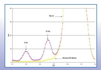
A major advantage for the MESA-7220 is the ability to analyze several elements in a single measurement. This spectrum illustrates the separation of Sulfur and Chlorine.
