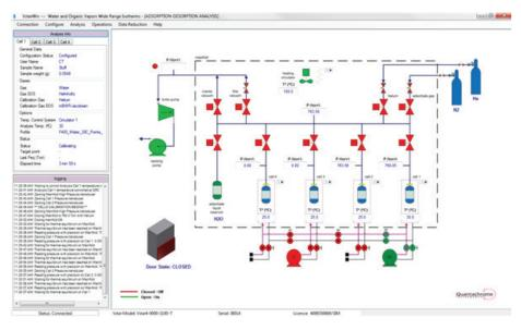
Intuitive dialogs allow programming flexible degas protocols and defining all acquisition parameters, from point selection to analysis temperature. Predefined protocols can be saved and used on a series of samples to ensure uniform analysis.
