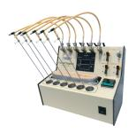
The FloVac provides cost effective vacuum degassing. Complete with single-zone heater (to 400°C), digital temperature controller and built-in digital vacuum gauge. Each sample station has its own adjustable evacuation / back-fill rate control. Flow degassing is also possible and can be advantageous in removing large quantities of moisture prior to vacuum degassing. Individual cooling stations. PC Temperature Control Software included.
