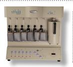
The gold-standard in sample preparation for physisorption analyzers. It provides PC control of all heating zones with individual heating ramps and times. The built-in cold trap enable efficient removal of condensables at low degassing temperatures and for a clean vacuum. Turbo- pumped version available for rapid high-vacuum degassing.
