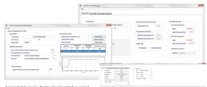
Acquired data can be displayed and printed or copied into reports and other documents. Basic data processing routines such as BET surface area and Dubinin-Radushkevich are built into the basic software.
