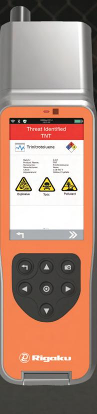
**Progeny ResQ** provides the power of Raman spectroscopy in a handheld form with no compromises. Users are empowered to choose the complexity of the task at hand. Progeny ResQ's unique software design provides articulate communication of simple threat identification for actionable decisions — for a variety of applications in the field or wherever data is needed.
