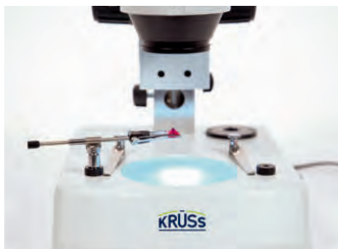
Figs. 35a (left) and 35b: Bright-field microscopy of a gemstone and schematic depiction of this illumination.
