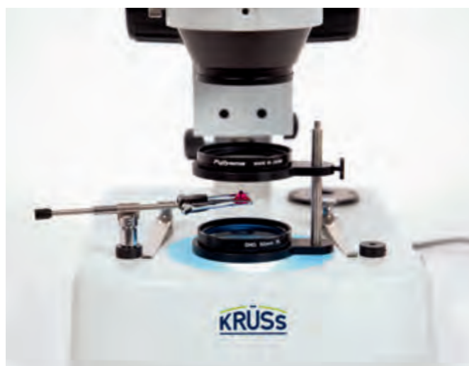
Figs. 36a (left) and 36b: Bright-field microscopy with polarisation units and schematic depiction of this illumination.
