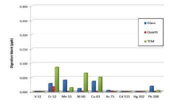
Figure 3 - Digestion blanks obtained from 2 different vial materials selected USP elements.
