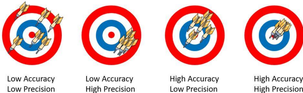
Figure 1: Diagram showing possible combinations of accuracy and precision. The cases with “high precision” provide better quality and process control.
