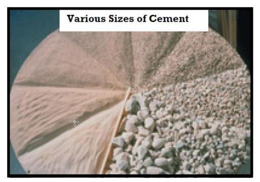
In addition, many studies have been conducted examining the relationships between Portland cement particle size distribution (PSD) and hydration and hardened paste strength properties. Within certain
