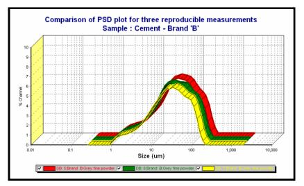
Above is a comparative graph of the three cement samples measured using the Turbotrac accessory on a Microtrac S3500. Notable is that Brands A and C are very similar but are different in distribution from Brand B. Brand B contains a larger percentage of coarser particles larger in size than 45 microns.
