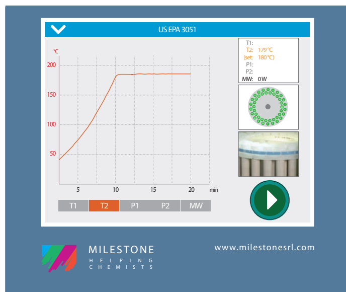
Temperature profile of a soil digestion in accordance with US EPA 3051 using the MAXI-44 rotor
