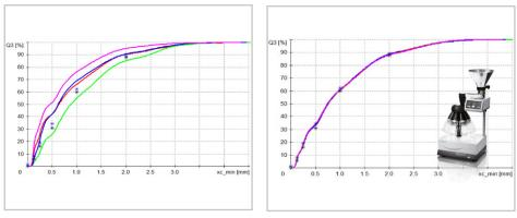
Fig. 1 (left): Random sampling. Four measurements with the CAMSIZER P4 image analyzer (red / blue / violet / green) provide four different results. None is within the expected range (black and blue \*).
