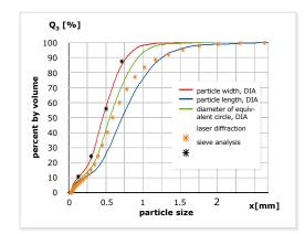
Fig. 5: Particle size distributions of a sample of coffee powder determined with sieve analysis (black \*), laser diffraction (orange \*) and dynamic image analysis. Image analysis provides three results based on particle width (red), particle length (blue) or circle equivalent diameter (green). The definition "width" fits well with sieve analysis, laser diffraction tends to correspond to circle equivalent diameter.
