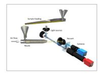
Fig. 2: The dry dispersion module of the CAMSIZER X2
