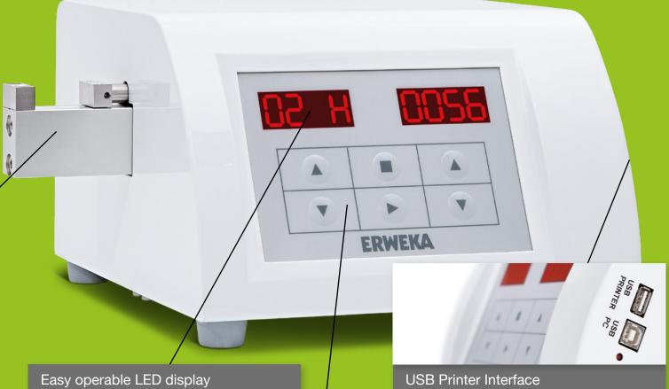
The test results (including date/time) are displayed on two LED screens in the following units: Newton (N), Kilopond (KP) or in Strong Cobb (SC).
