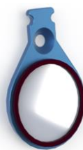
Fig. 40: Calibration filter: the lens with specified tint must reflect the value (end value) \pm 3\%
