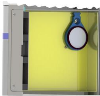
Fig. 39: Sample collection receptacle with inserted calibration filter
