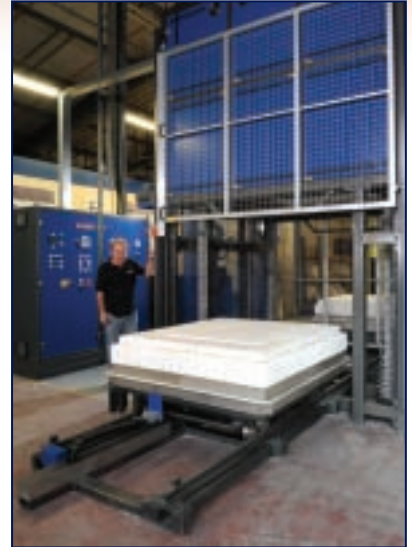
DUAL BOGIE RAISED HEARTH FURNACE FOR RAPID BATCH CHANGES
