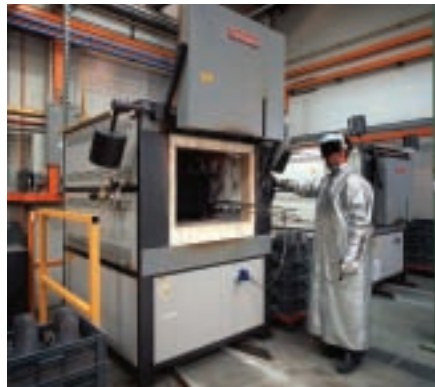
LARGE CAPACITY 1200°C FURNACE WITH MODIFIED ATMOSPHERE RETORT
