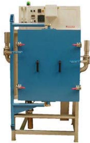
A Custom Designed Oven for Curing Silicone Hydrogel Contact Lenses
