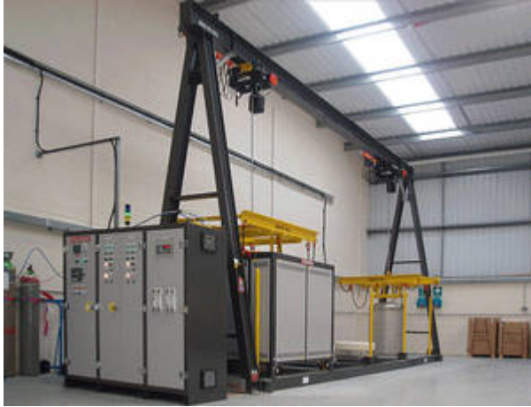
Dual-hearth Top Hat Furnace System
