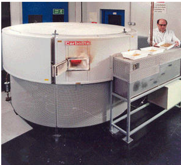
Rotary Hearth Furnace
