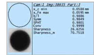
Image of a spherical metal powder particle
