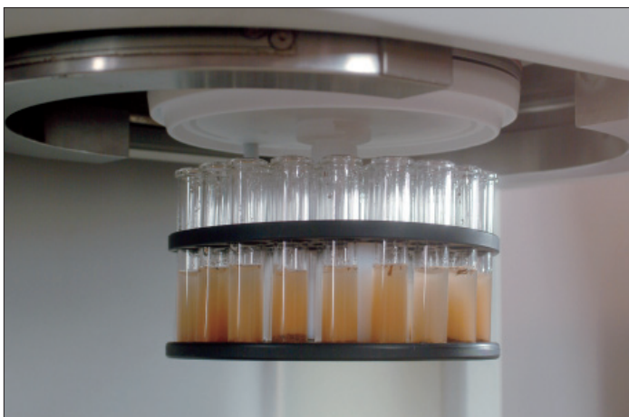
PHOTO: A 40 position rack in position prior to digestion. The SRC chamber will rise up from below and be locked in position by the two clamps.
