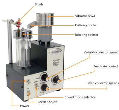
The **Rotary Micro Riffler**<sup>™</sup> easily and automatically divides samples into eight(8) smaller representative samples for analysis. By repetitive divisions of the collected smaller samples, the desired final sample size can be easily obtained.
