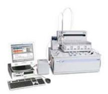
Flow Injection Analysis (FIA) and Ion Chromatography (IC) are complementary analytical techniques that are commonly used in the same laboratory. The QuikChem® 8500 Automated Ion Analyzer offers an Ion Chromatography Option to complement its basic FIA capability. By incorporating both technologies into a single instrument, the following benefits are achieved:
