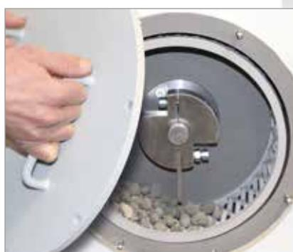
Closing the filled grinding chamber
