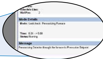
The Mode Details give you the status of the current leak check.
