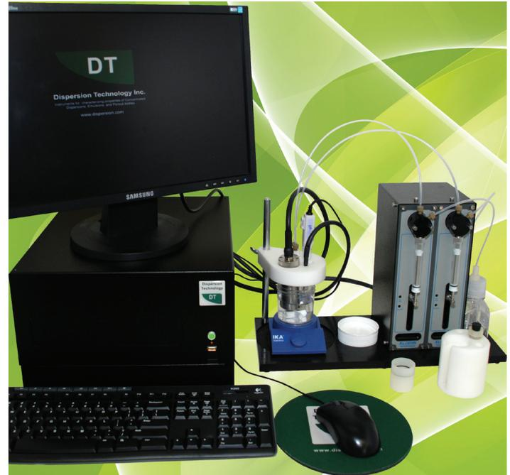
Models DT-300 and DT-310 have a unique **Electroacoustic sensor**, which is built as a probe (see on the right) for measuring  $\zeta$ -potential in concentrates without dilution. The same probe can be used for monitoring sedimentation kinetics.
