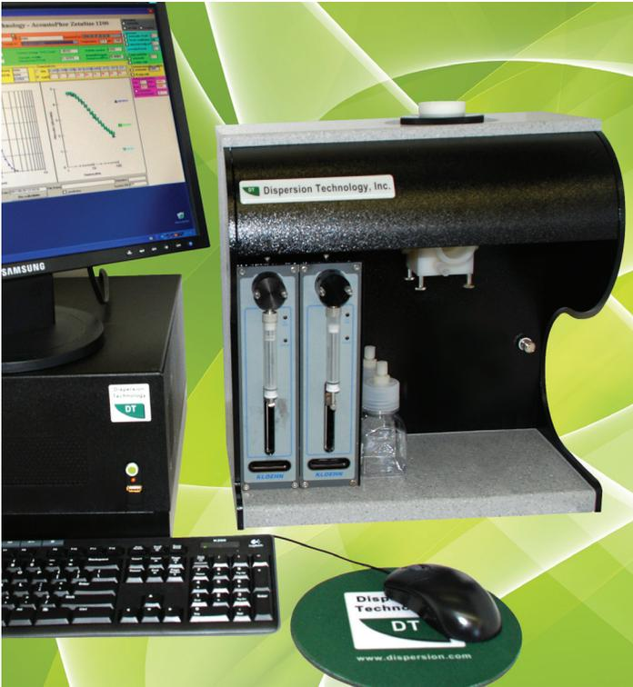
Model DT-100 has a unique Acoustic sensor for characterizing *particle size distribution* by measuring ultrasound attenuation at set of frequencies from 1 to 100 MHz, as well as sound speed. This method can be referred to as “*ultrasound scattering*”.
