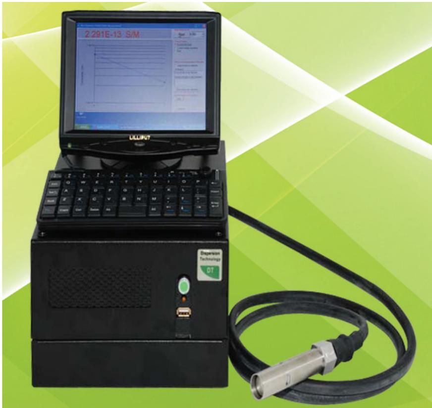
**Model DT-700** is a stand alone instrument for measuring electric conductivity of low polar (alcohols) down to completely non-polar liquids (toluene, hexane, etc) within the range of 7 orders of magnitude. This measurement can be used for studying ionic composition of such liquids, which affects many properties of the liquids, emulsions and dispersions. Consequently, this instrument is suitable for the quality control of these properties.
