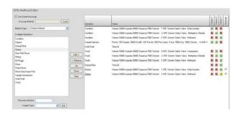
This example method is more complicated and shows the real flexibility of the PrepLinc™ software. Three SPE columns are used for this example. Condition and wash steps are performed to move the sample through all three columns. A reverse elution is performed on one of the columns for the final collection. Both elutions are evaporated using the optional AccuVap™ and can be collected in separate vials.
