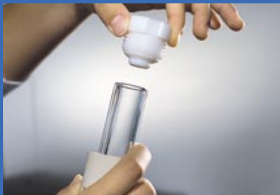
Q-20 vessel components
