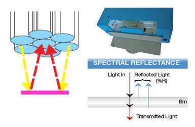
The reflected light is collected and the light interference created by the deposit is processed by a spectrometer. The software analyzes the interference fringes and calculates the deposit thickness.
