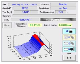
Until 2014, only the visual rating method was used for specification purposes but it was suffering from the drawback of operator subjectivity. ASTM decided to use SI unit to report the result of the jet fuel thermal oxidation deposit. Following this decision, the DR10 – ITR became referee method.
