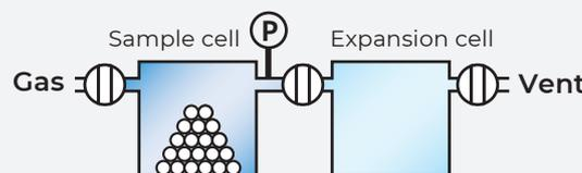
Pressure is measured after He is introduced to sample cell.
