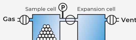
Gas is diffused into expansion cell when opening the valve and pressure is decreased. The sample volume is measured from the change in pressure.
